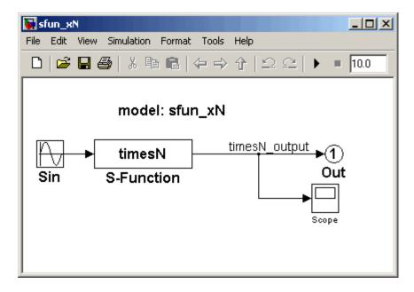
**4** View the previously generated code in sfun\_xN\_grt\_rtw/sfun\_xN.c. Note that no loops exist in the code. This is because the input and output signals are scalar.
