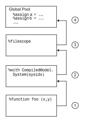
The rule for nested file scopes is similar to that for nested function scopes. In the case of nested file scopes, only the innermost nested file scope is searched.
