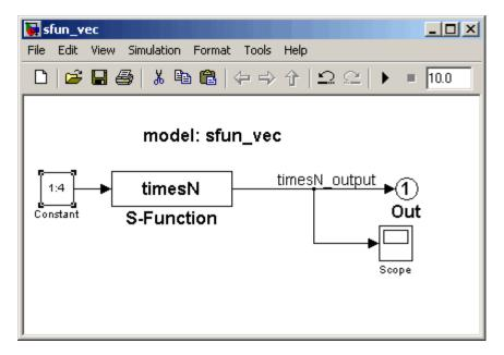
4 Because the Constant block generates a vector of values, this is a vectorized model. Generate code for the model and view the /\*Model output function \*/ section of sfun\_vec.c in your editor to observe how variables and for loops are handled. This function appears as follows:
